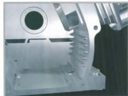
Cooling Fins inside Crankcase
